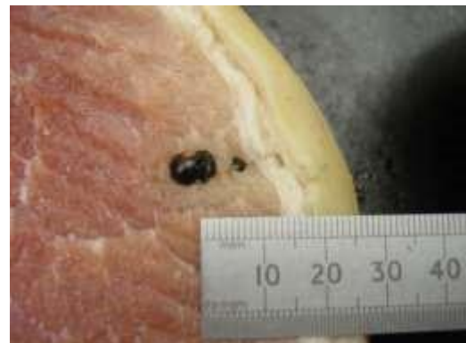
6mm BB (plastic) Impact velocity: 1232 FPS (840 MPH) Impact energy: 8.22 joules Pellet weight: 1.8 grains Result: Penetration to 18mm
