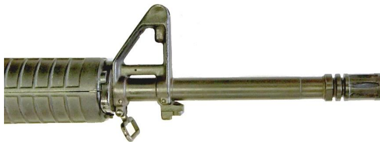
Pic 7 5.56mm rifle with flash hider attached
