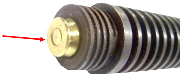
Pic 8 .45 ACP Thompson 1928A1 barrel, the actual barrel length is shorter than the length the "rod down the bore system" gives.
