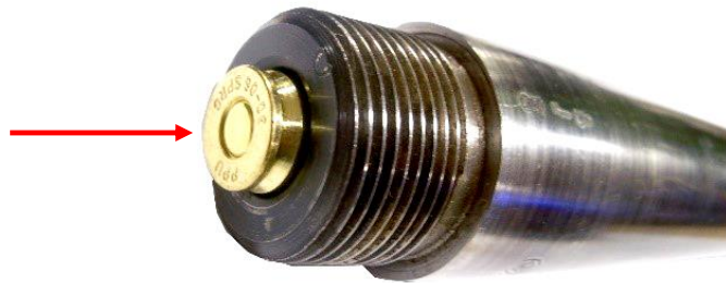
Pic 10 30-06 Winchester Model 70 Sporter barrel, the actual barrel length is shorter than the length "rod down the bore system" gives.
