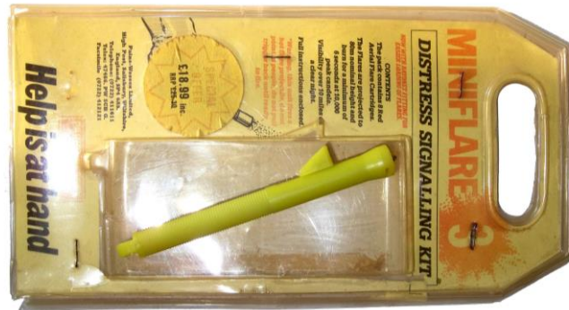
Pic 6 Compact distress signalling mini flare MK8 using a spigot type mechanism and a centre fire shot gun primer to ignite the propellant (lab exhibit A20311)
