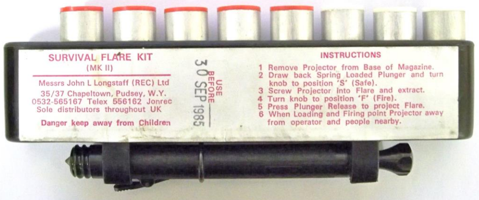
Pic 8 Spigot type compact distress signal mini flare kit using a spigot type mechanism and a centre fire shot gun primer to ignite the propellant (lab exhibit 251)
