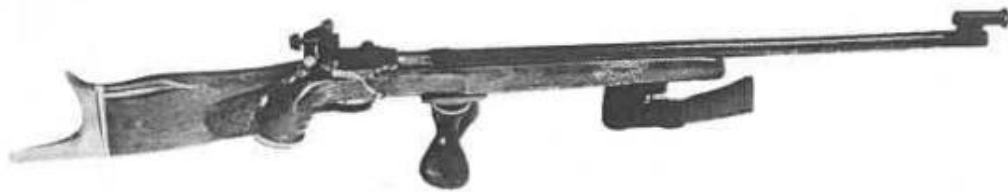
A Dr. M. K. Jurek 22 LR single shot match rifle. This rifle incorporates his own design of bolt action operated by pulling the handle to the rear which retracts the bolt by means of a toggle action. The receiver is marked "patent pending". Floating heavyweight round barrel with sight dovetail at muzzle, rearsight dovetail at left of action, adjustable trigger and special walnut stock with dovetail slide for adjustable buttplate, large finger grooved pistol grip with thumb hole, cheekpiece and adjustable handstop, palm rest for offhand shooting, alloy hand stop, tunnel aperture foresight, fully adjustable rearsight with camera type adjustable iris diaphragm.
