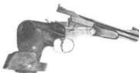
Action open, the Model 5 gun reveals it is solidly constructed, with deep and full fit in the length of the frame. Jurek guns, as target arms, do not eject the fired shell, but simply lift it portaway out of the chamber.
