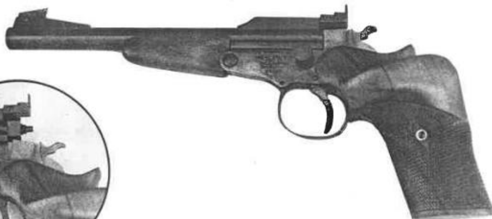
This .360 caliber muzzleloader is owned by the author. It was, in fact, made for him. The design differs from the Model S only in that the receiver is cut away to permit the percussion nipple to seat itself in the same position a centerfire cartridge primer would occupy. Thus, the action breaks for nipple-seating and a nice straight-line ignition path is provided.
