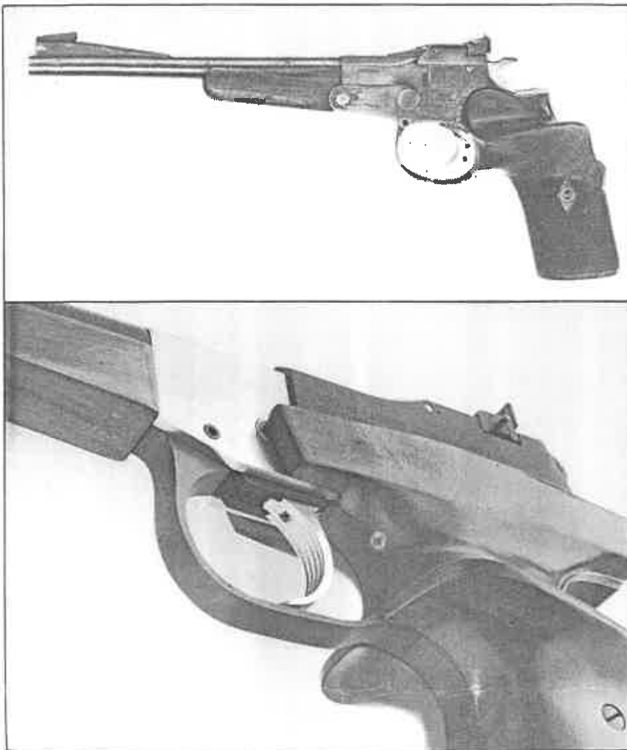
Left: A typical break-barrel model 'Popular', the owner of this gun felt the need for a trigger shoe.
