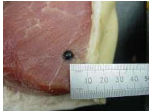
6mm BB (plastic) Impact velocity: 1066 FPS (726 MPH) Impact energy: 6.17 joules Pellet weight: 1.8 grains Result: Penetration to 9mm
