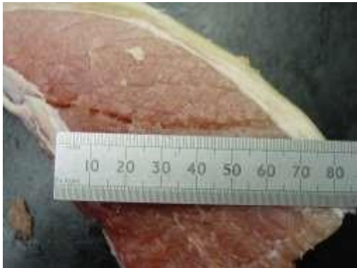
.177 BB (Steel) Impact velocity: 719 FPS (490 MPH) Impact energy: 8.25 joules Pellet weight: 5.3 grains Result: Penetration to 70mm
