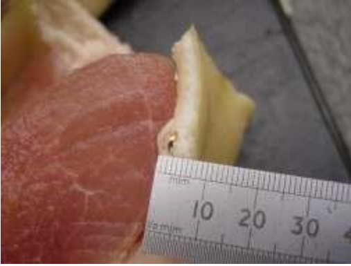
.177 BB (Steel) Impact velocity: 413 FPS (281 MPH) Impact energy: 2.72 joules Pellet weight: 5.3 grains Result: Penetration to 3mm
