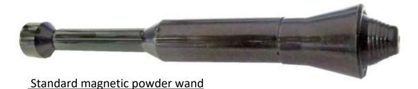
The wand has a magnetic stem, allowing magnetic powder to be collected and brushed over the desired surface. The magnet can then be released by extending the spring-loaded handle, in order to drop the powder after use. The outer casing is plastic to allow for easy cleaning; therefore the wand can be used with a variety of different colours of magnetic powder.
