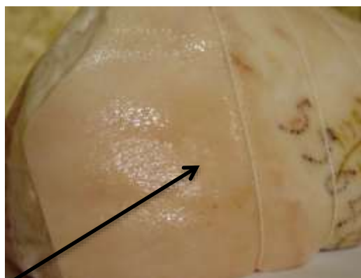
6mm BB (plastic) Impact velocity: 657 FPS (448 MPH) Impact energy: 2.43 joules Pellet weight: 1.8 grains Result: No penetration
