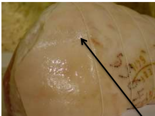
.177 BB (Steel) Impact velocity: 243 FPS (165 MPH) Impact energy: 0.95 joules Pellet weight: 5.3 grains Result: No penetration
