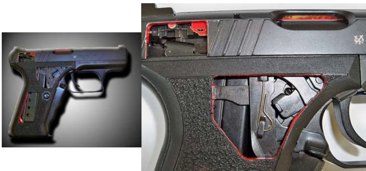
Heckler and Koch 9mm pistol Model P7 M8. Produced 1979-2008. Semi automatic pistol fitted with "squeeze cockling lever", 8 round single stack magazine.
