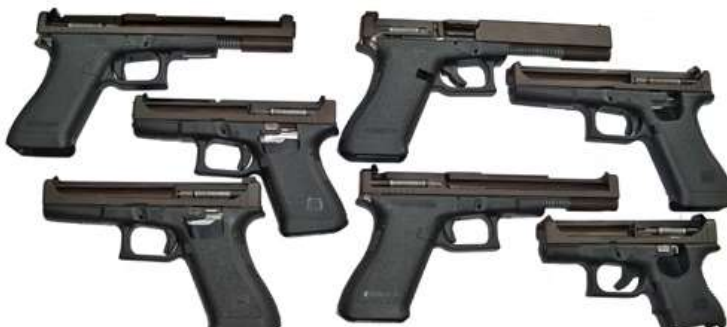
Glock Pistols (cutaways) used to demonstrate action function and the effects of miss matching components.
