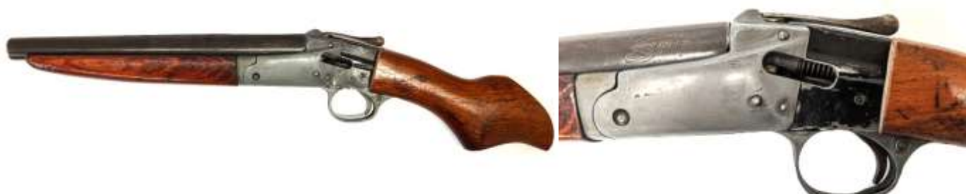
12 bore single barrel BSA shotgun. An example of the 'in line' firing pin.
