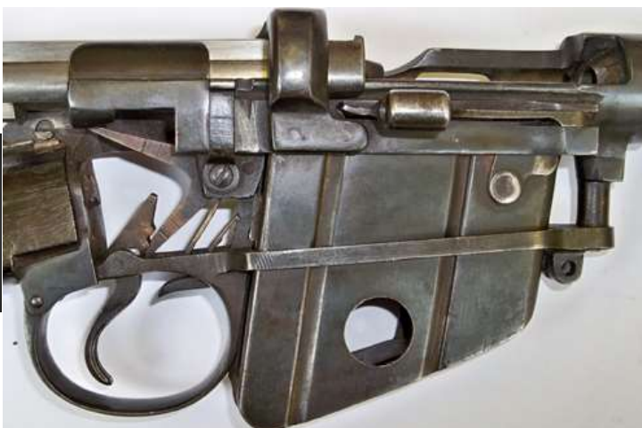
Short magazine Lee Enfield MK111 (SMLE) 1907, used in WW1. This original cutaway model was used to train armourers. Filled with mag charger bridge and mag cut off.
