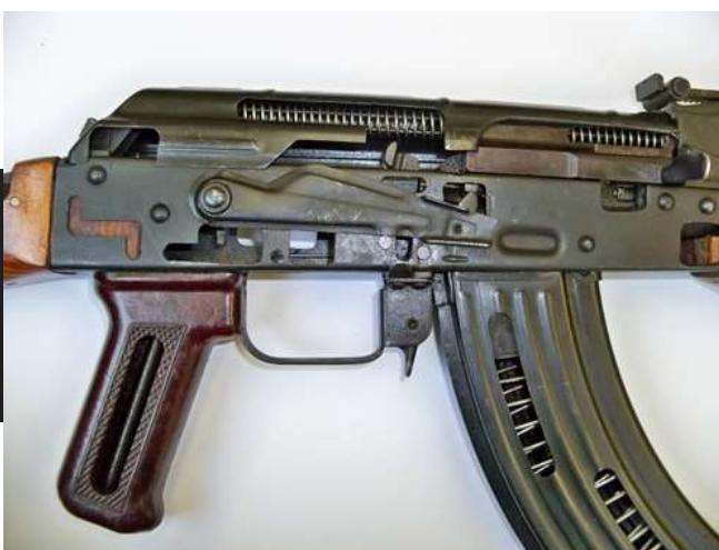
AKMS of unknown manufacture, chambered for 7.62x39mm. Long stroke gas action with semi-automatic/ fully automatic trigger mechanism.
