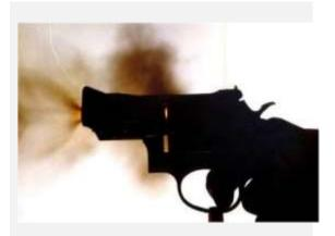
Muzzle blast. The dangers from particles of propellant, wads, restrictors, etc. leaving the muzzle at high speeds are very real. Safe distances must be established and enforced
