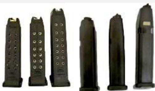
9mm magazines showing modifications over the years, followers are also updated to enable the pistol to function with the latest ammunition designs
