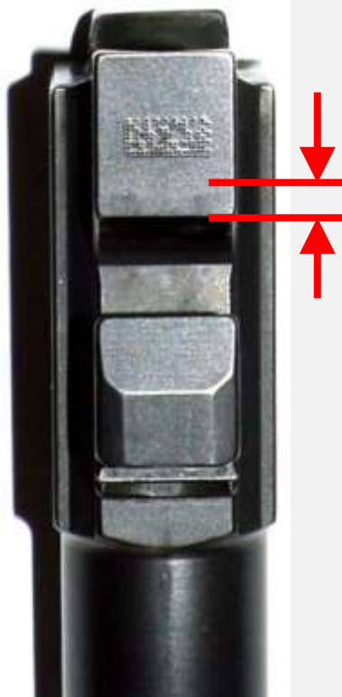
Barrel showing contact between barrel and locking block
