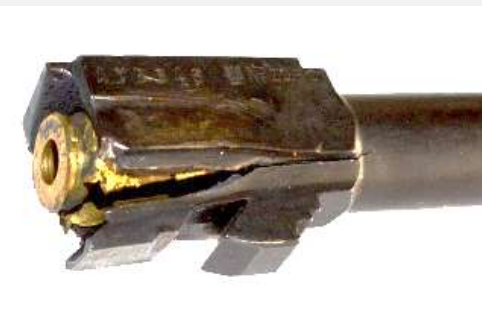
"Breech explosion" in a 10mm barrel
