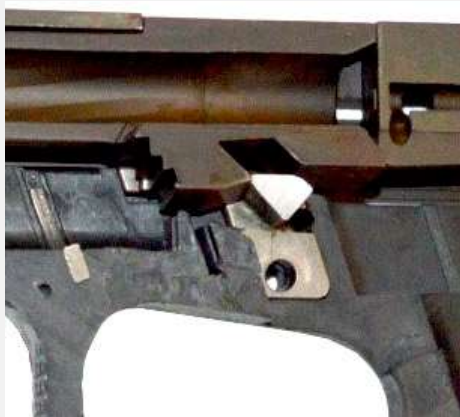
Locking contact between the locking block and barrel
