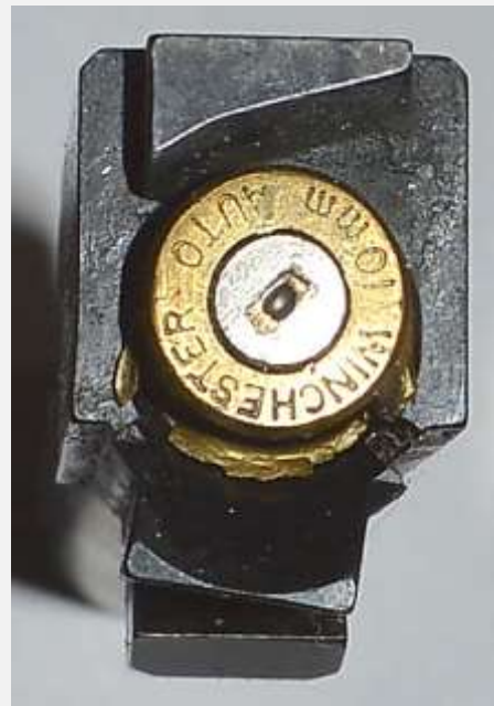
The effect on a cartridge case due to high pressure, causing the barrel to fail
