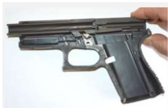
Examining the locking block function and areas of contact with the barrel, when the pistol is in battery
