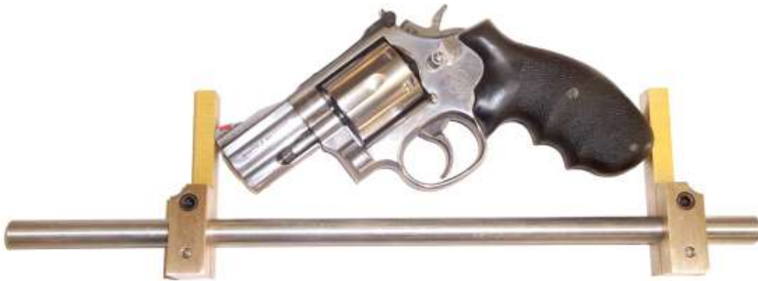
Pic 1 Overall length measuring system
