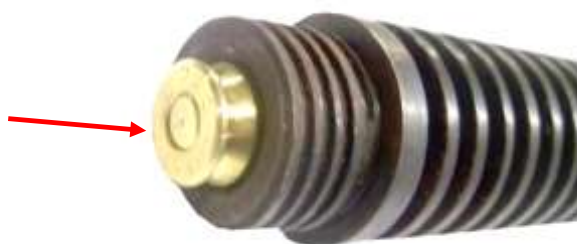
Pic 8 .45 ACP Thompson 1928A1 barrel, the actual barrel length is shorter than the length the "rod down the bore system" gives.
