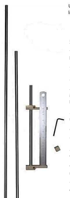
Used for accurate overall measurements covering lengths of interest in the Firearms Acts.
