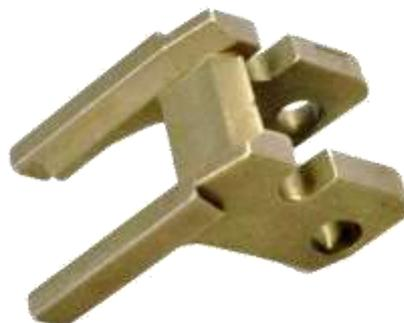
15] The locking block's function is to bring the barrel into battery as the slide moves forward into the firing position. The block cams the barrel into position and the top of the locking block holds the barrel firmly into battery, the two locking surfaces shown below.
