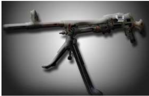
FN mag 58 Belgian manufactured, general purpose machine gun, designed in the early 1950's and used by more than 80 countries. Calibre 7.62x51.
