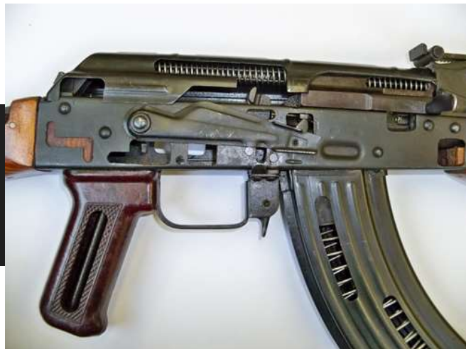
AKMS of unknown manufacture, chambered for 7.62x39mm. Long stroke gas action with semi-automatic/ fully automatic trigger mechanism.
