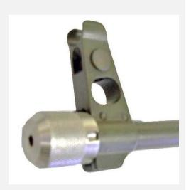
Matching the blank firing attachment to the blank you use is a must, too much recoil can damage the receiver beyond repair
