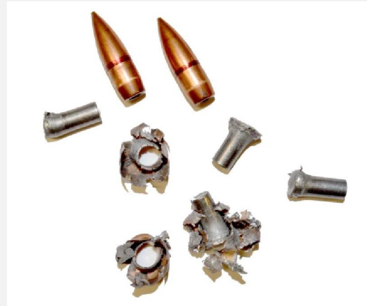
AK47 steel core bullets before and after hitting the new material AA processed as shown above
