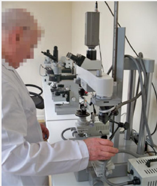
Matching bullets to the gun that fired them requires the use of a comparison microscope
