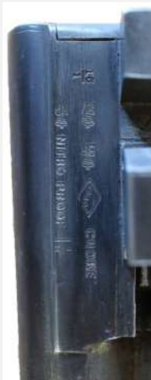
Proof marks on a shot gun barrel
