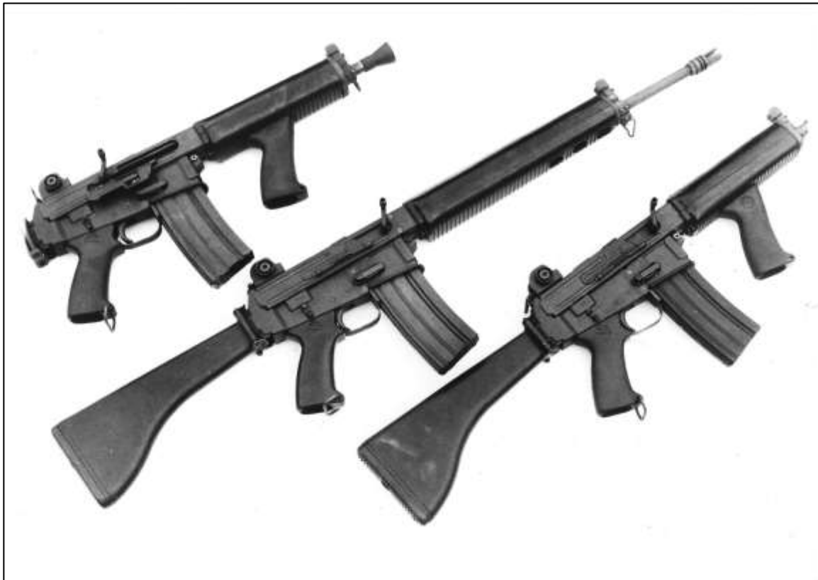
AR-18S w/o stock (left), AR-18 (center), AR-18S (right, muzzle cropped in original photo). Note shorter AR-18S barrel length.
