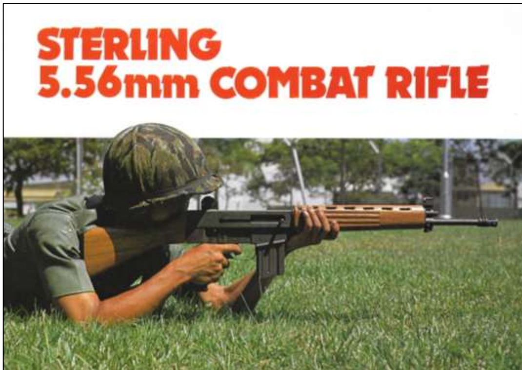
Early CIS prototype Sterling Combat Rifle with wood furniture circa 1978. With assistance from Sterling the wood was soon replaced with plastic furniture.
