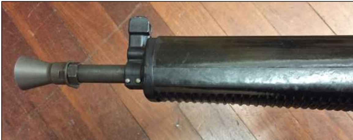
Production Sterling AR-18S (AS063) with 1-inch longer barrel (courtesy UK Defence Academy).
