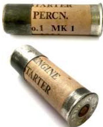
Pic 4 Blank cartridges designed to be used to start engines
