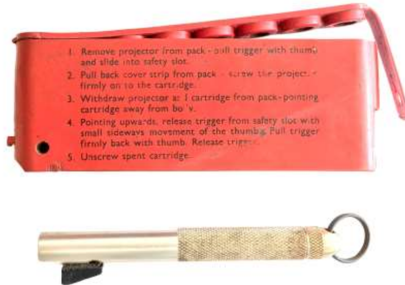
Pic 1 Mini flare kit and launcher (lab exhibit SP7855)
