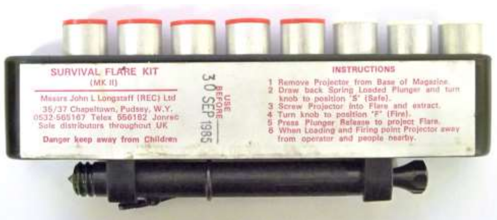
Pic 8 Spigot type compact distress signal mini flare kit using a spigot type mechanism and a centre fire shot gun primer to ignite the propellant (lab exhibit 251)
