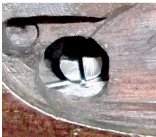
Trigger free play on sears (with safety disengaged)
