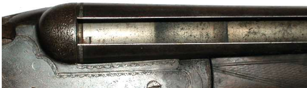
Deposits left after firing a 2" RTO cartridge in a 2 3/4 " chamber
