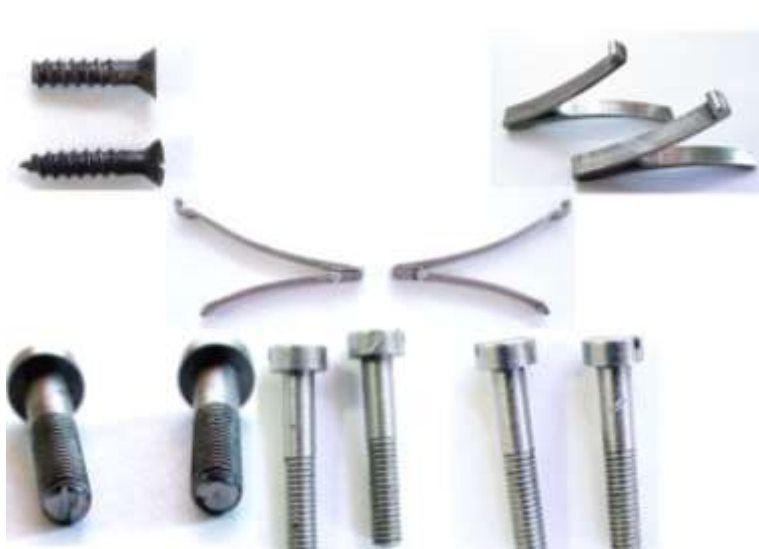
Left hand screws and springs normally have a mark
