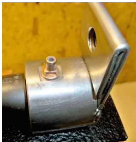
Pic O7 Beryllium Copper nipple fitted
