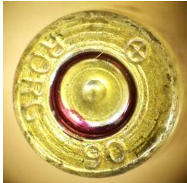
Pic 12 Cartridge case and primer impact marks against the test barrel breech face after firing
