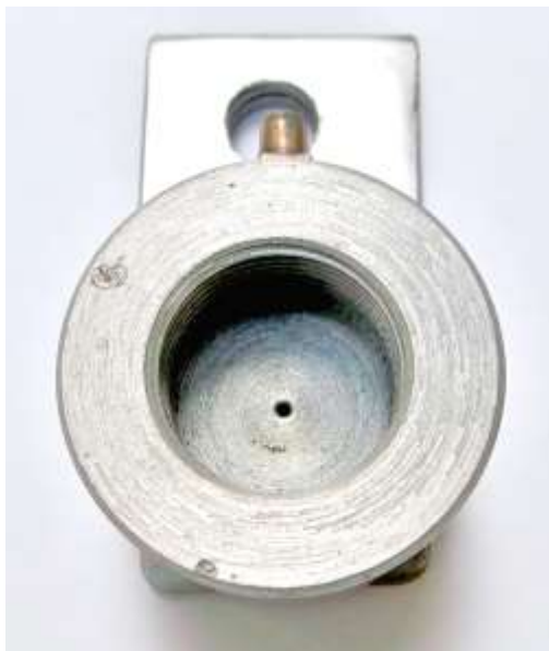
Pic O5 Breech Face with firing pin hole
