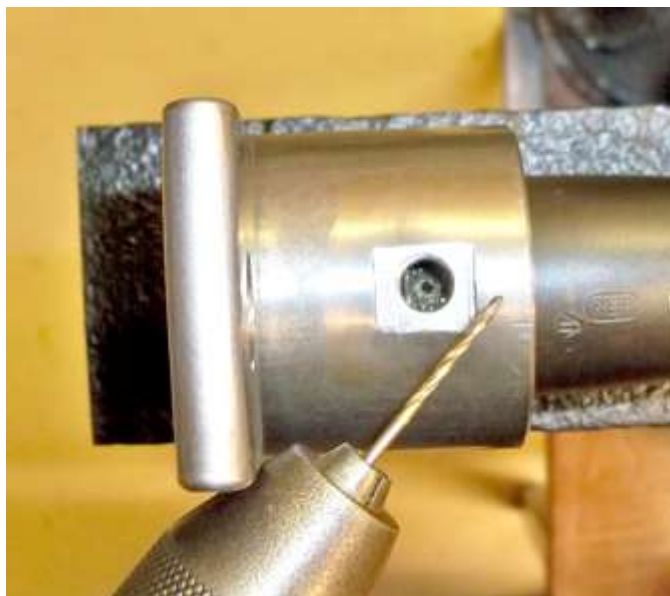
Pic O6 Breech face fitted to the barrel ready for drilling flash hole
