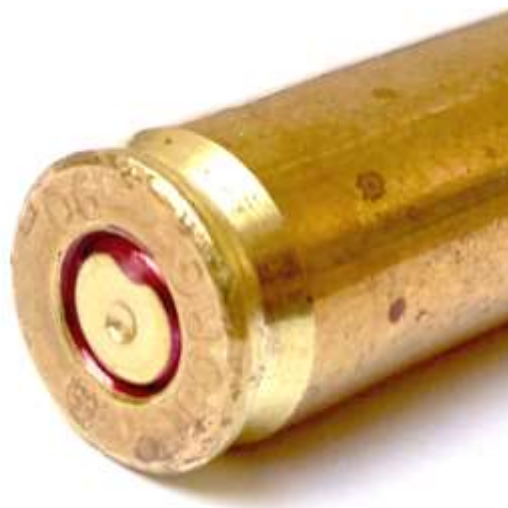
Pic 03 Reloaded round with fired primer
