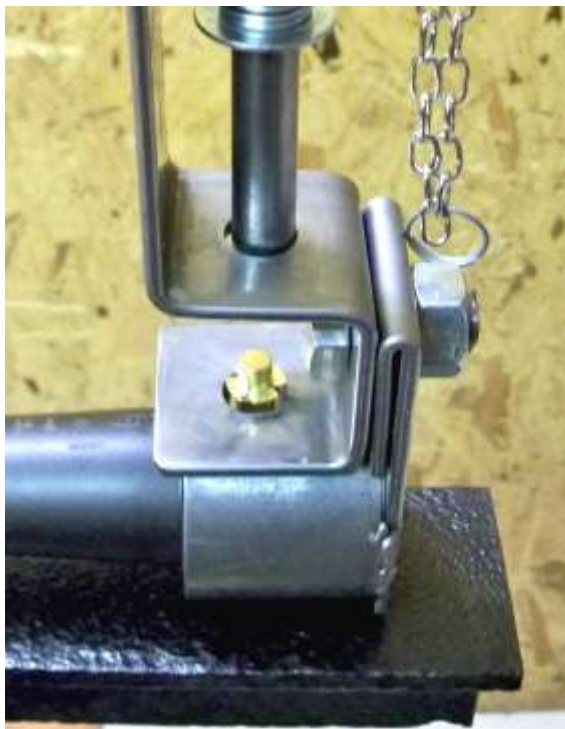
Pic 09 Firing mechanism fitted with a military type percussion cap in place, cartridge case drilled to allow the flash of the percussion cap to ignite the propellant
