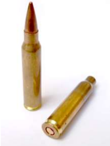
Pic 01 Complete L2A2 round and case with unfired primer
