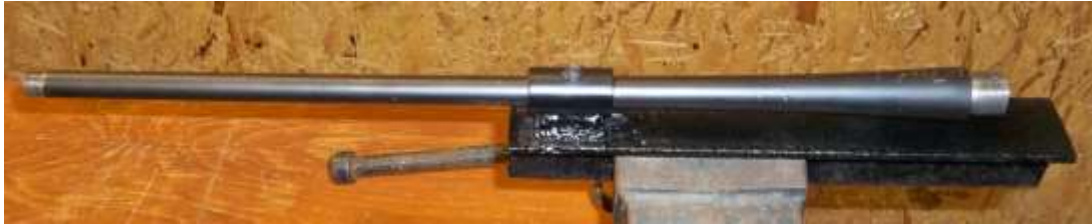
Pic O4 test barrel fixed to test bed
