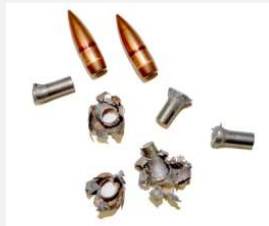
AK47 steel core bullets before and after hitting the new material AA processed as shown
