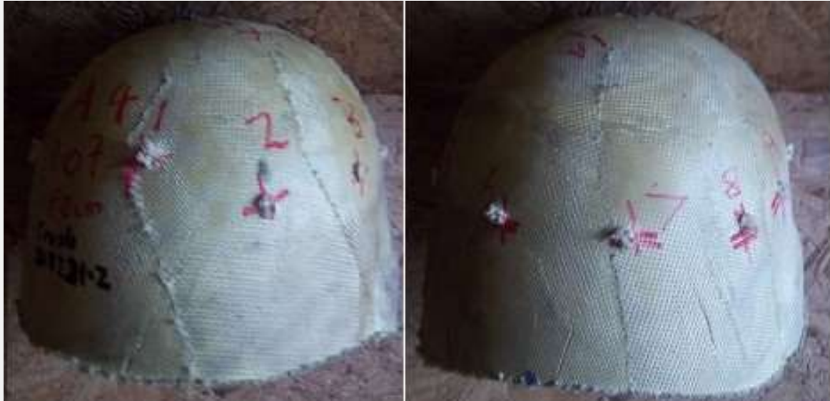
Helmet Shells front (left) and rear (right) showing Fragment Simulated Projectiles (FSP) impacts during V50 (ballistic limit) testing
