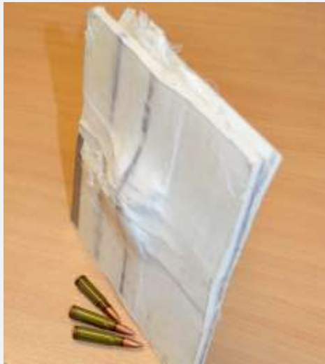
UMNPE materials (AA processed) offer a lightweight solution for stopping the AK47 steel core bullet
