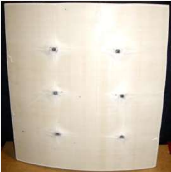
UHMWPE Plate stops AK47MSC and M80 Ball at 12mm
