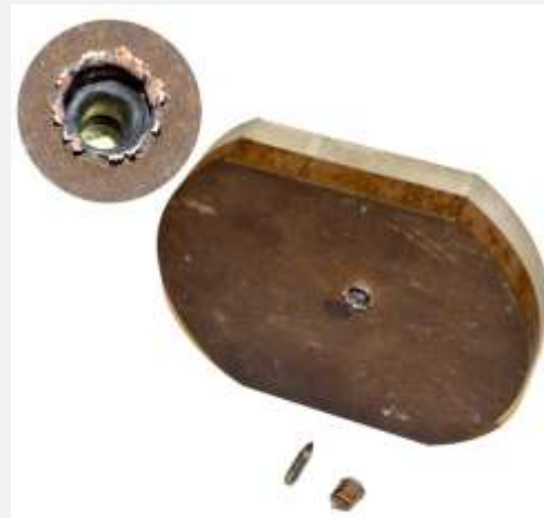
30 mm thick steel and alloy material unable to stop the M2AP bullet
