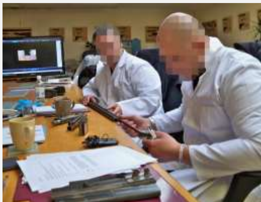
Shot gun barrel dimensions are taken to accurately record the correct choke dimensions, prior to pattern testing with a range of ammunition types
