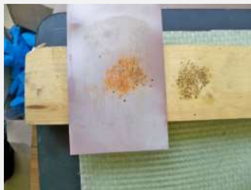
Reverse modified grease test for non-porous materials, the picture shows the 'lift' taken from the sample deposits on a wood post
