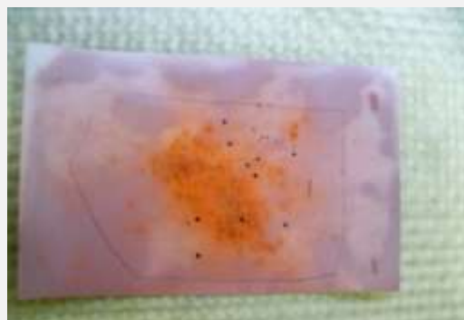
Modified grease test showing nitrites and evidence of un burnt propellant (nitrates)
