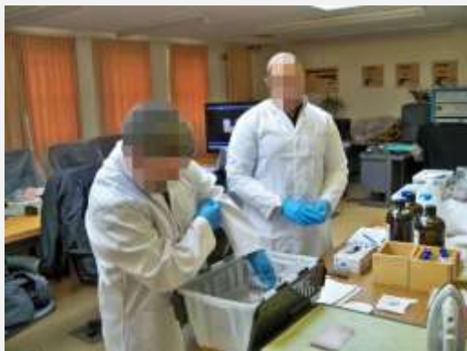
Dipping the nitride free material in acid solution, used to lift nitrides from the suspect clothing
