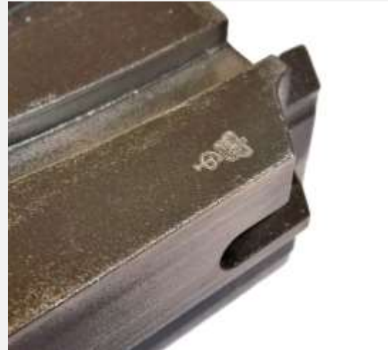
Where components have been replaced remember the major components require to be proofed
