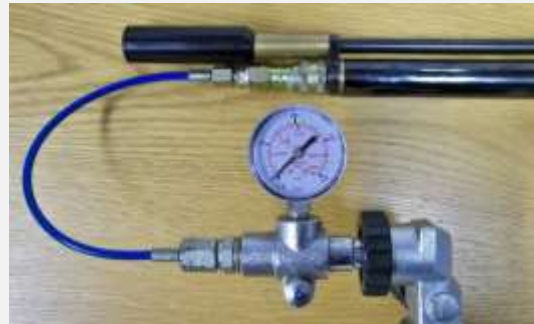
Charging the P.C.P as per the manufacturer's instructions
